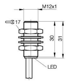
Inductive Sensors BES 516-375-E4-Y M12x1 x 33 normally-closed Sn=2mm shielded
